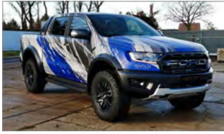
Wrapped by Foliateure, Germany. Printed film: OS-500 White Wonder - Laminate: OS-510 Razor Blade
